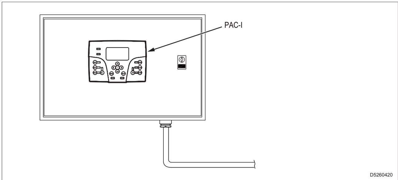
The generating set combined with a PAC-I mains/generator switchboard, forms a complex for the supply of electricity within a few seconds from the sudden absence of the commercial electricity grid.
