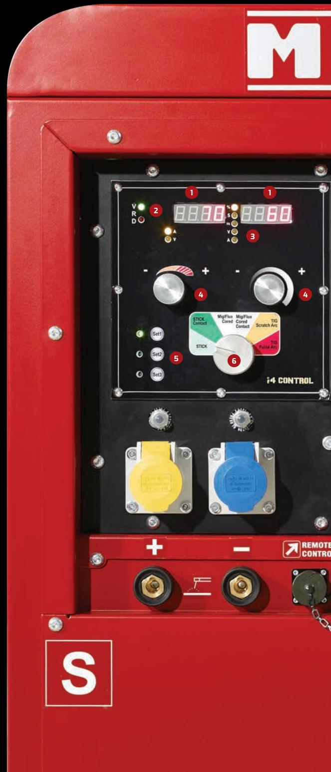
The front panel of the new series TS EVO MULTI4 focuses on all the control functions of the engine driven welder. Controls and indicators are set out in a clear, rational way ensuring quick and easy selection of welding parameters by the operator.
