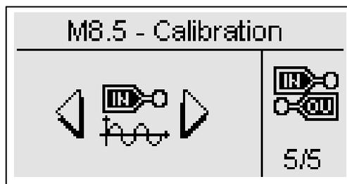
The measures setup allows to adjust the measured values for genset and mains voltages and load currents. For each voltage measure it's possible to set a calibration offset with steps of 0.1 V. For each current measure the offset is a percentage of the CT ratio, in steps of 0,1 %.
