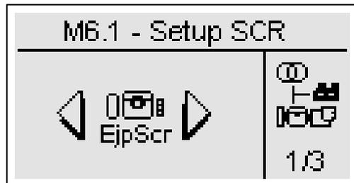
It permits to start the generator by a remote signal on one of the programmable inputs, that you have to set to remote start (see par. 2-10). When that input is closed to negative, after a START BY SCR DELAY time, the generator starts. Then:
