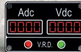
Welding DSP Voltmeter/Ammeter
