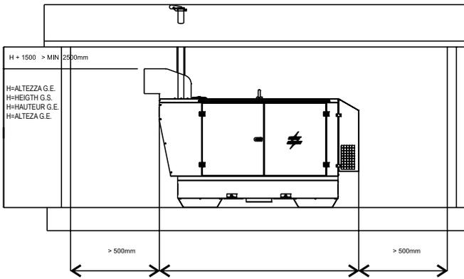
Floor should be levelled and suitable to sustain genset weight. Thresholds on doors and openings should have a barrier in order to avoid liquids leaking. In case it is not possible to provide a door with a barrier, the genset should have a collection base appropriate for the quantity of liquid it contains, in any case dimensions of collection base must be in accordance to the laws in force in country of installation.
