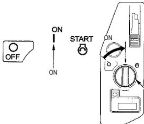
5) Turn the engine switch to the ON position.
