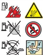
Gasoline is highly flammable. Refuel with motor shut off in a flat surfaced well-ventilated area. Do not refuel in the presence of flames. Avoid spilling fuel. Any eventual spilled fuel and fumes are flammable. Clean any dispersions of fuel before starting up the motor.
