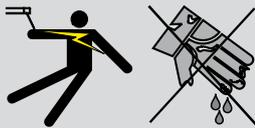
Do not use the machine with wet or damp hands and / or clothing. Use plugs suitable for the output sockets of the machine and make sure that electrical cords are in good condition.
