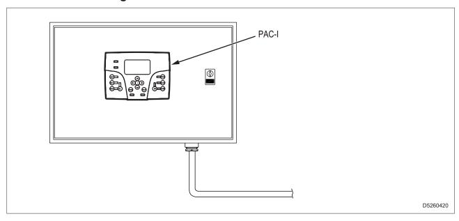
The generating set combined with a PAC-I mains/generator switchboard, forms a complex for the supply of electricity within a few seconds from the sudden absence of the commercial electricity grid.
