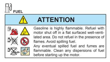
Fill the tank with gasoline for automobiles (preferably lead free or with low lead content in order to reduce deposits in the combustion chamber to a minimum).
