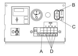
In case of emergency due to engine failure, or due to failure of the hydraulic or the electrical system, use the bypass tap of the solenoid valve to lower the mast. When the mast is completely down, close the tap again.
