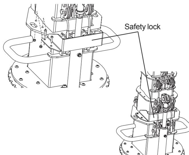
The safety lock stops the lowering of the mast at a safe height. This avoids the risk of operator injuries in the event of sudden failure of the telescopic mast ropes or the hydraulic lifting system.
