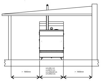
Floor should be levelled and suitable to sustain genset weight. Thresholds on doors and openings should have a barrier in order to avoid liquids leaking. In case it is not possible to provide
