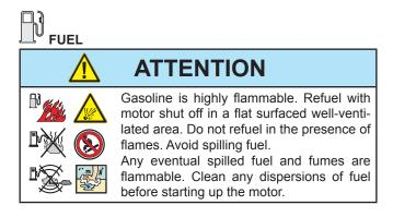
Fill the tank with gasoline for automobiles (preferably lead free or with low lead content in order to reduce deposits in the combustion chamber to a minimum).
