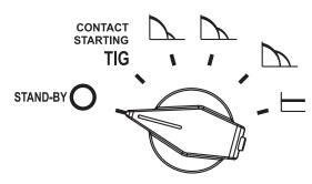
There is a manual switch for selecting the various welding processes on the welding control panel.
