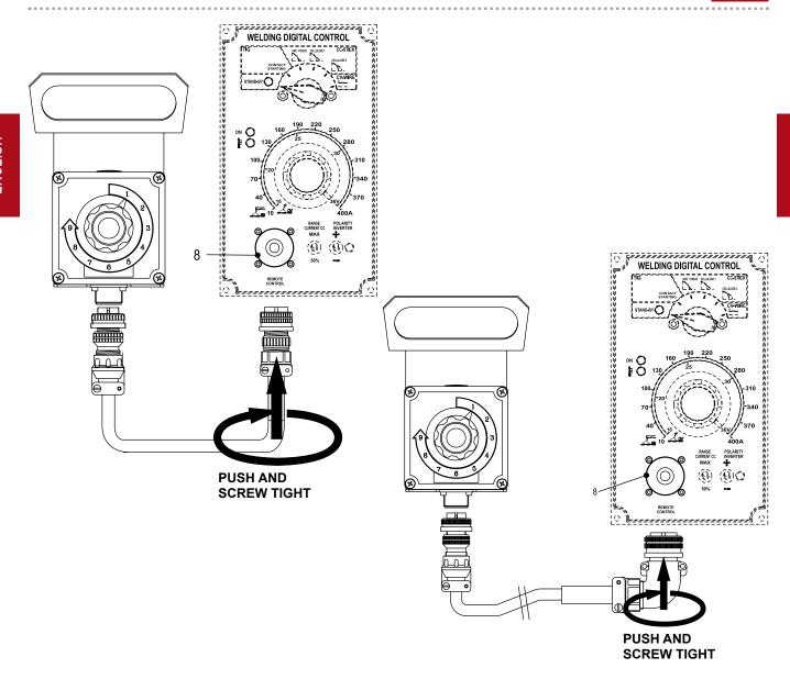
The remote control RC, which regulates the welding current in the CC (STICK welding) mode and the welding voltage in the CV (MIG/MAG welding), is connected to the front panel by means of a multipole connector.
