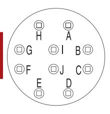
Put the knob on RC1 at minimum/max, put one ohmmeter from pin A - B and measure the resistance.
